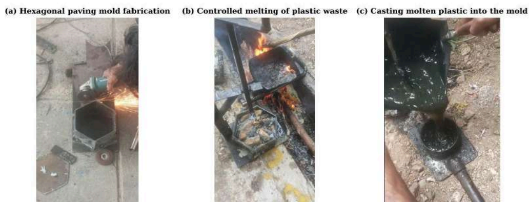
Figure 3. Paving mold fabrication and the controlled melting/casting process: (a) hexagonal paving mold fabrication; (b) controlled melting of plastic waste; (c) casting molten plastic into the mold.
