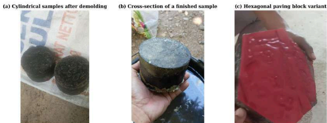
Figure 4. Upcycled paving block samples obtained after demolding: (a) cylindrical samples; (b) cross-section of a finished sample; (c) hexagonal paving block variant, later subjected to the quality tests in Section 4.3.
