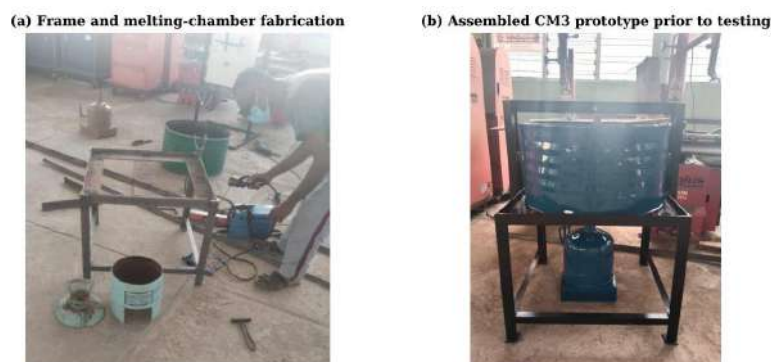
Figure 2. Design and fabrication of the CM3 prototype: (a) frame and melting-chamber fabrication; (b) assembled CM3 prototype prior to testing.
