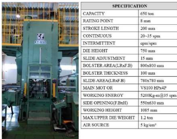
Figure 4. Vertical 650T Forging Machine and Specification
